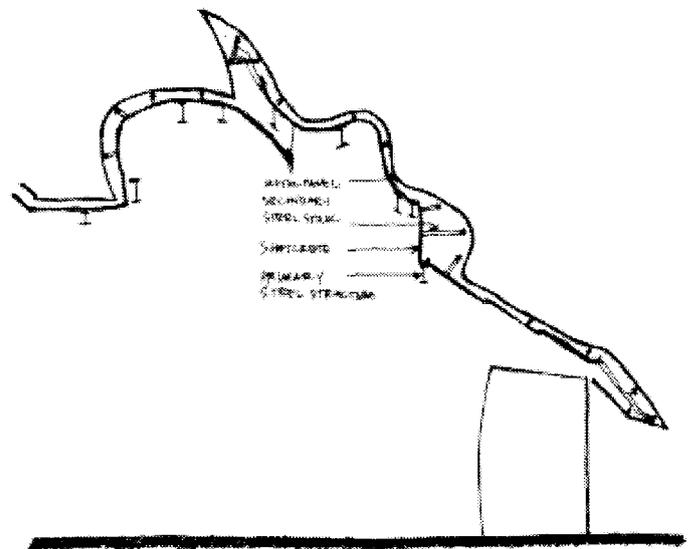
Figure 1. Section Diagram of EMP's structural and cladding system
